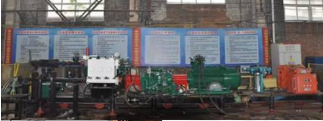
Test and Test System for 10KVA High Pressure Mine Pump
